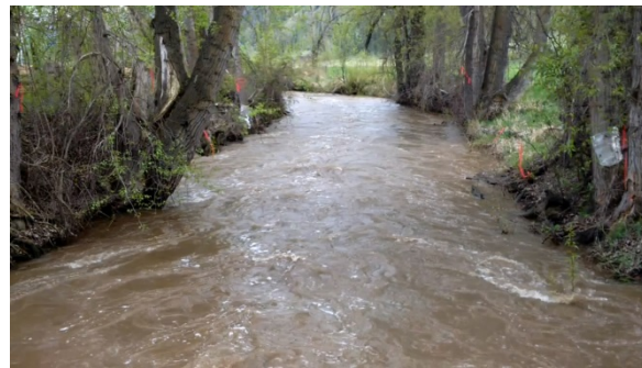
Video from bridge: Field of view includes both banks, control points not well defined
